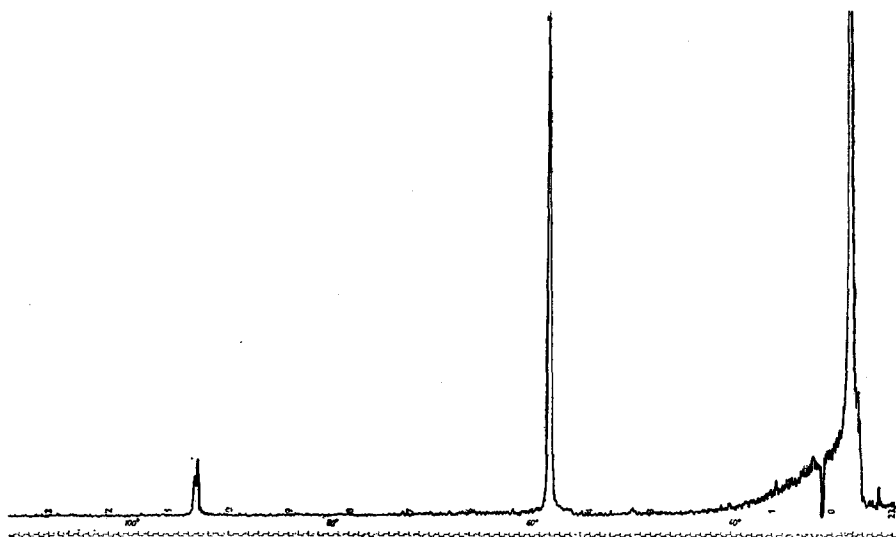
Figure 3.3. A Bragg diffractometer recording of a film of 20 mol % GeTe and 80 mol % PbTe on glass substrate.
