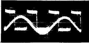
Fig. 35. Waveforms of anode current and cathode heating current ( p=10^{-4} torr, U_a=50 V, U_a=50 V, I_f=45 A).
